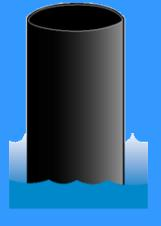
All Black Used to mark one side of a well defined channel. Go between it and its companion "all red" spar buoy
