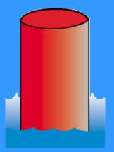
All Red Used to mark one side of a well defined channel. Go between it and its companion "all black" spar buoy
