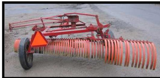
**This road rake is traditionally towed behind a truck or a road grader to remove rocks but is too wide to be used on many dirt roads and has been known to remove a crown rather than create one...**
