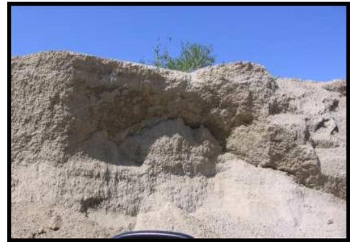
Another way is to see if it flows freely under the tailgate of the haul truck when the driver attempts to “tailgate spread” by hooking the tailgate chains to the body to only allow a certain amount of gravel to run out under the tailgate gate as he drives along. If it does not come out, it probably has good binder, though the truck driver will be quite annoyed at having to break loose the bound up gravel from behind the tailgate before he lengthens the chains!
