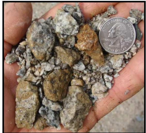
¾" minus crushed gravel with fines washed out so the larger "aggregate" is visible. Note the sharpness of the stone due to this being ledge based gravel and that the stone is approximately the same size as a quarter
