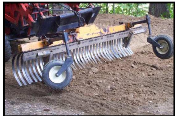
**Grading and backblading to obtain final shape**
