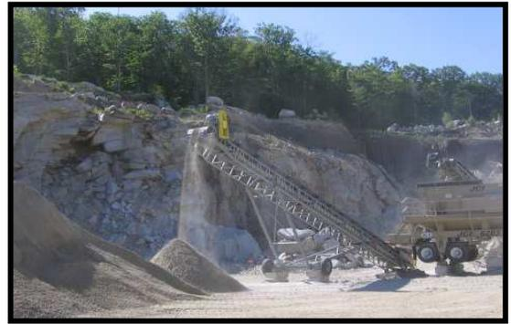
**Besides producing "aggregate" that is uniform in size and, ideally, in content of fines versus stone, this process makes stone that is much more angular than that made just from screening bank-run gravel**
