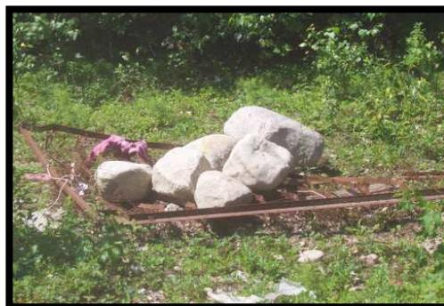
While a drag of this type does help to redistribute material, it does little to cut to the bottom of potholes, reclaim material from the shoulder, separate accumulated debris, or restore crown. In fact, indiscriminate use of a
