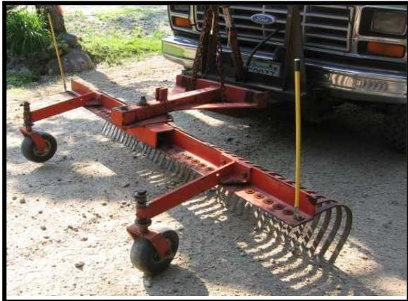
**This tractor style three point hitch rear mounted landscape rake was retro-fitted to the plow hoist of a truck as a low cost alternative to a FrontRunner. While it does not have power angling and is not as rugged as the Front Runner, it can perform regular maintenance duties without the owner having to have a tractor solely for that purpose and has the added advantage of being *ahead* of the operator.**
