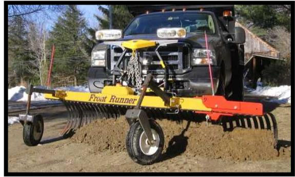
The **FrontRunner** grader/rake mounts in front of a truck in place of the snowplow and uses the snowplow controls to feather, lift and angle it.
