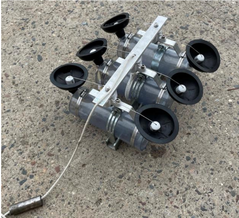
Figure 16. SAFL-built Van Dorn water sampler that instantaneously captured three one-liter samples at a selected water depth.
